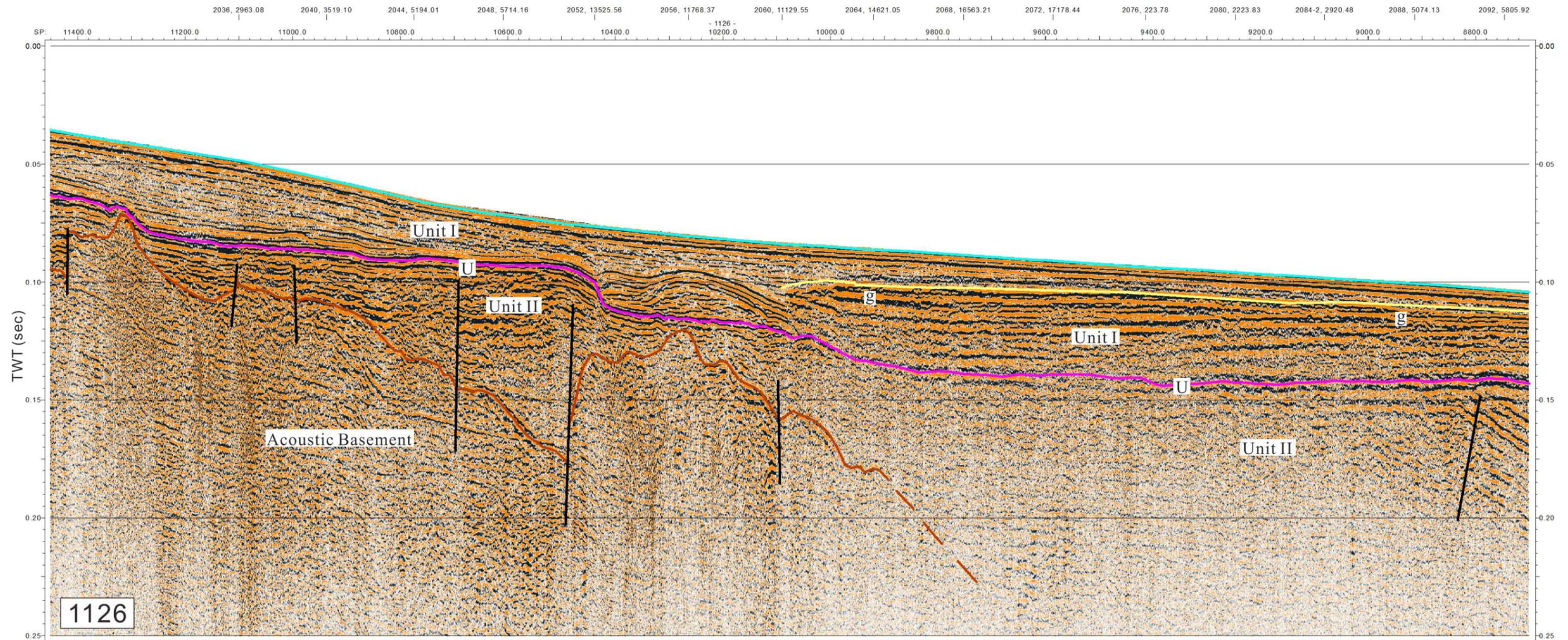
—U— : Unconformity    / : Fault    g : Gas Charged Sediments
