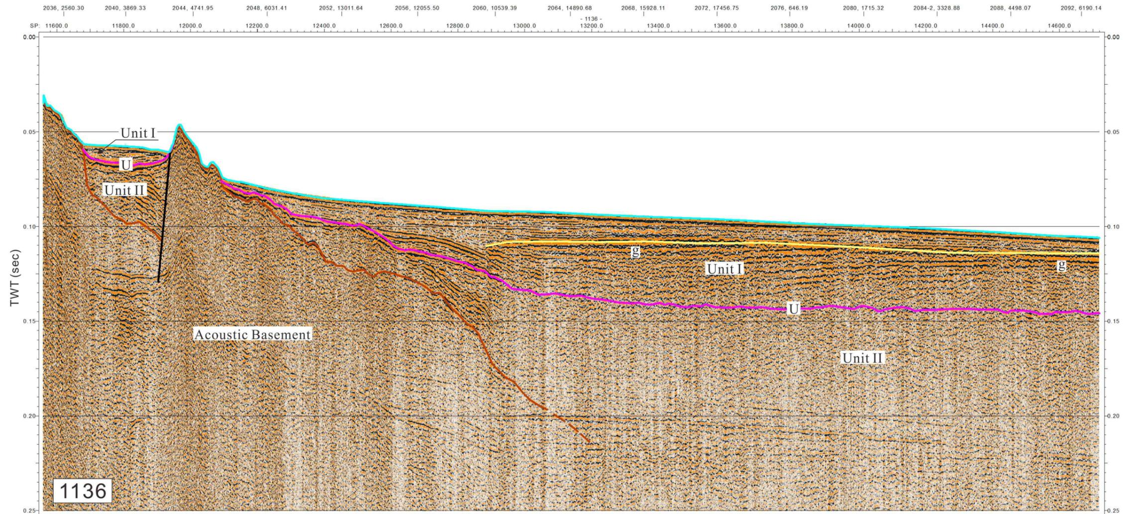
—U— : Unconformity    / : Fault    g : Gas Charged Sediments
